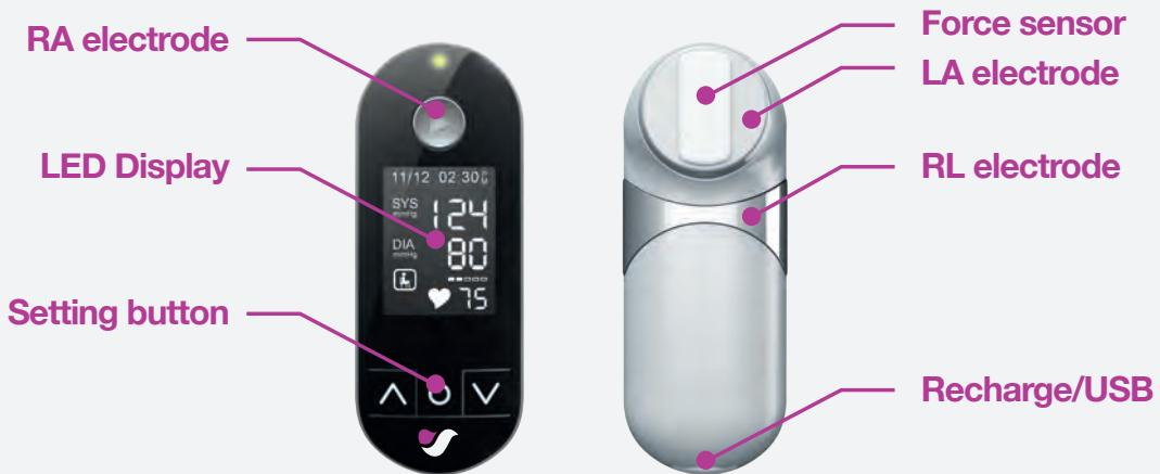
The device senses the lead 1 ECG and radial artery pulse by using 3 electrodes and 1 force sensor. With these bio-signals, the device gets certain parameters, including pulse transmission time (PTT), and calculates Systolic and Diastolic Blood Pressure according to a formula. The devices can also calculate heart rate (HR) and indicates irregular heart beat as well. To get both the ECG and pulse bio-signal, the user have to
