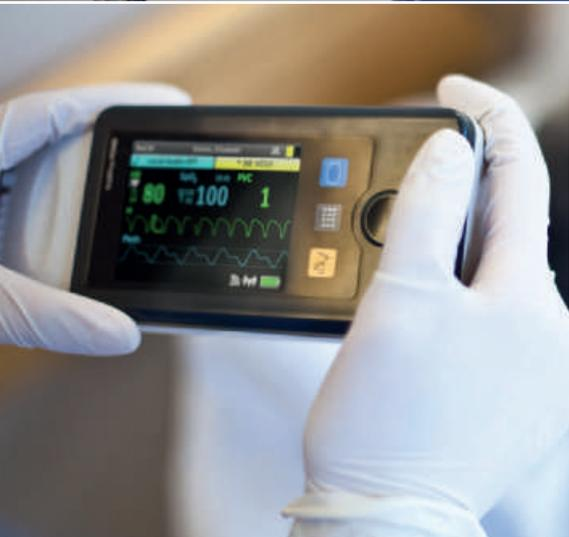
The color touchscreen display “sleeps” to conserve battery and provide patient privacy, yet can be activated with the touch of a button. A display lock allows viewing and is designed to avoid making unintentional changes.
