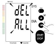
2. Press the "S" button to confirm deleting and the LCD will display "dEL dOnE", and then turn off.
