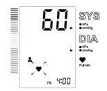
2.Press the "START/STOP" to power off, otherwise it will turn off within 1 minute. Display and save the results.
