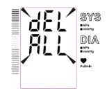
2.Press "SET" button to confirm deleting and the LCD will display "dEL dOnE", and then turn off.
