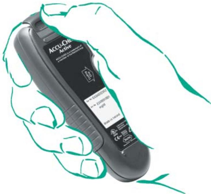
A new battery provides enough power for about 1,000 tests. When you first see the battery symbol displayed, there is still enough power for about 50 tests, though we recommend that in this event you replace the battery as soon as possible. By then the battery will have been considerably drained, and changeable conditions (cold surroundings) can affect its performance even further.
