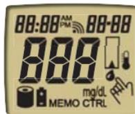
This is a display check. If any parts or number segments are missing or unclear, call the ACCU-CHEK Customer Care service center at **1-800-858-8072**.
