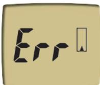
The test strip was bent or removed during testing, or the measurement window cover is not on correctly.
