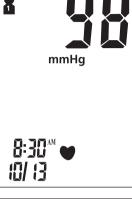
4. When testing is complete the monitor will sound three short beeps. The screen will display your systolic and diastolic blood pressure. The reading will be automatically stored in the selected memory zone.
