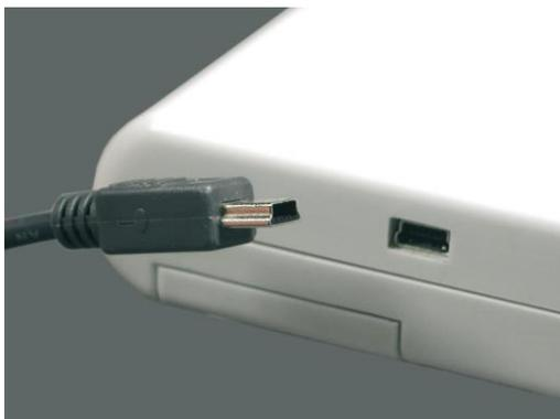
Figure 7: Connection of the Mini-USB cable
