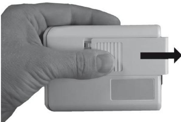
Figure 4: Opening of the battery compartment
