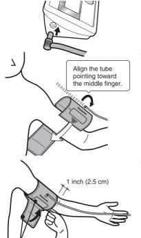
1. Insert the plug into the socket all the way in.
