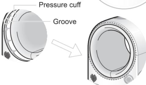
\* When re-attaching, be sure not to touch the inside of the main body where the pressure cuff has been removed. Doing so may result in an accident or injury.
