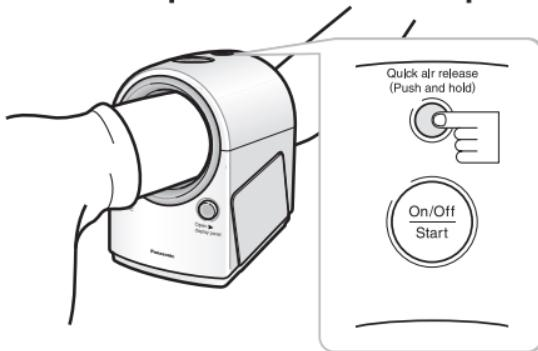
If the pressure cuff will not deflate even if the On/Off Start button is pressed, press the Quick air release button and hold it pressed. The air will be released in approximately 4 seconds.
