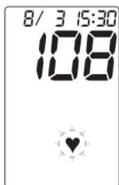
The heart mark ♥ will blink when pulse is detected during pressurization.
