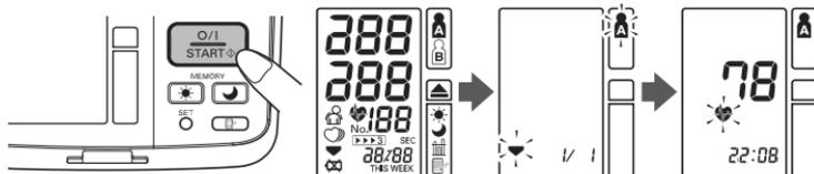
**Note:** To stop the inflation or measurement, press and release the O/I START button. The unit will stop inflating, start deflating and will turn off.
