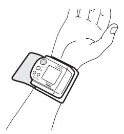
**Note**: attach the monitor upside down for reliable measurement at your right wrist.
