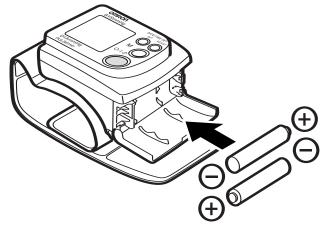
2 Insert two batteries in the battery compartment.
