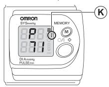
1 Press Memory Recall button to turn on power. Note: Display shows alternately blood pressures and heartbeats.
