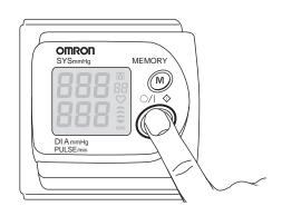
2 Press Memory Recall button for latest and previous values. Press On/Off button to turn off power.
