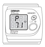
**1** Read the values of blood pressure and pulse from the display. **Note**: Display shows alternately blood pressures and heartbeats.
