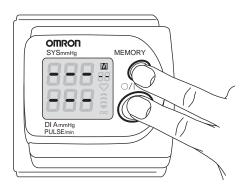
2 Press Memory Recall button and simultaneously On/Off button to erase memory.Caution! All stored values will be erased!Press On/Off button to turn off power.
