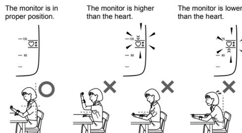
After the Positioning symbol lights for more than 2 seconds, the wrist cuff will start to inflate automatically.
