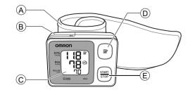
A. Wrist cuff B. Battery compartment C. Display D. Memory (冒) button E. START/STOP button
