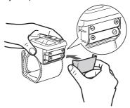
Make sure their polarity (+/-) is aligned with the polarity (+/-) as indicated in the battery compartment.
