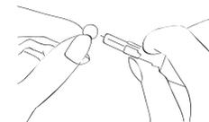
Replace the lancing device cap. Turn the cap until it is snug but not too tight.
