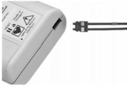
To download a monitoring plan or upload data, ABPM-04 has to be connected to the computer. Connect the small plug at the end of the twin optical cable into the socket on the bottom of the device (the cable indicated with red should be closer to the edge of the device). Insert and push gently until it clicks into place. The plug can be properly connected in one direction only.
