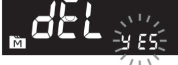
To delete all the results, press Main button and “yes” and “” are displayed on the meter, press SET to delete the memory.
