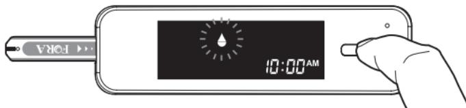
1. Start with the meter switched off. Insert a test strip to turn on the meter. The screen will display a “” .
