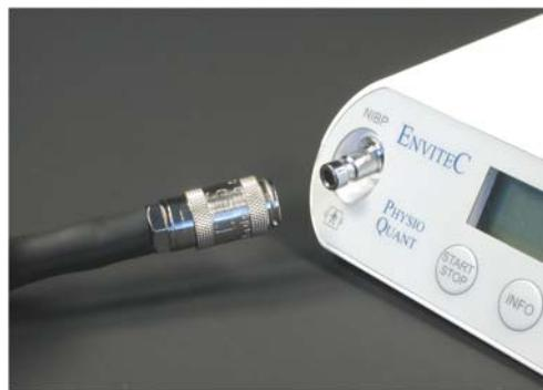
To connect the blood pressure cuff to the recorder, plug the metal connection of the cuff as far as possible into the connection point at the recorder, until it clearly clicks into place.
