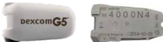
Figure 2. Dexcom G5 Mobile Transmitter Front and Back
