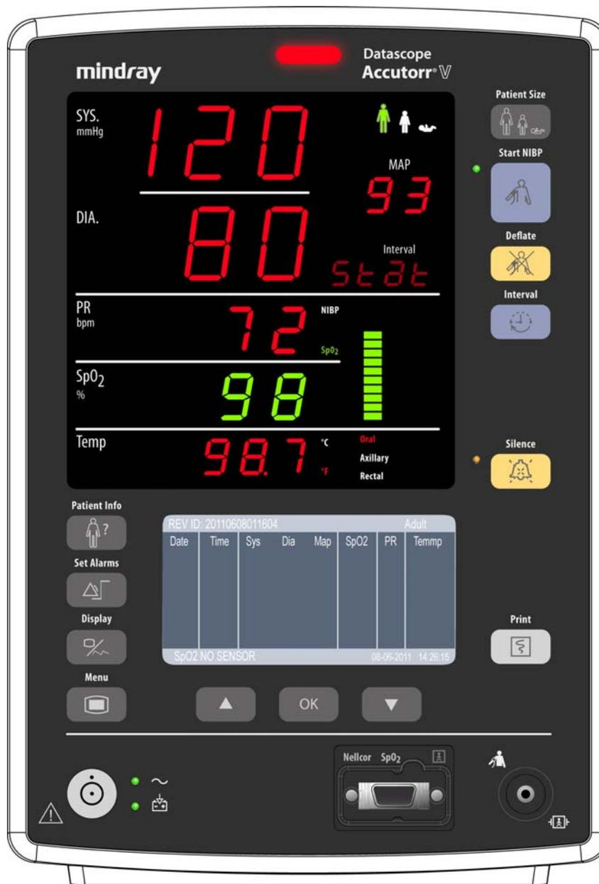
**FIGURE 1-1** View of Accutorr V Front Panel
