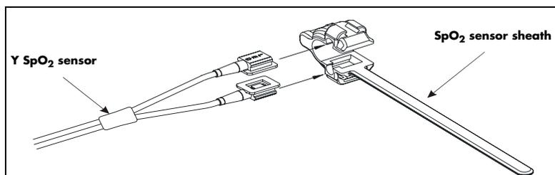
**FIGURE 3-17** Inserting the Y SpO<sub>2</sub> sensor into the sheath
