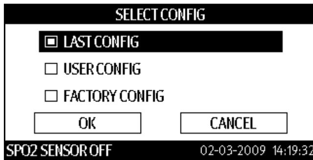
**FIGURE 3-29** Default Power-on Configuration Selection Dialog (SELECT CONFIG)
