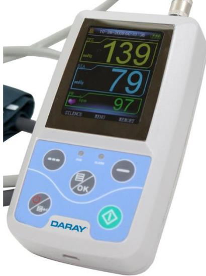
For the convenience of operation, the different interfaces are on different parts of the monitor. At the top is the Socket for the SpO<sub>2</sub> Sensor and socket for NIBP cuff. At the bottom is the USB socket
