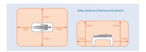
Without medical safety devices, e.g. medical protector, the PC and all the non-medical devices connected to the system (e.g. monitor and printer), must be set up and used at a distance of at least 1.5 m to the patient unit (see the orange area in the figure), as leakage currents can occur.
