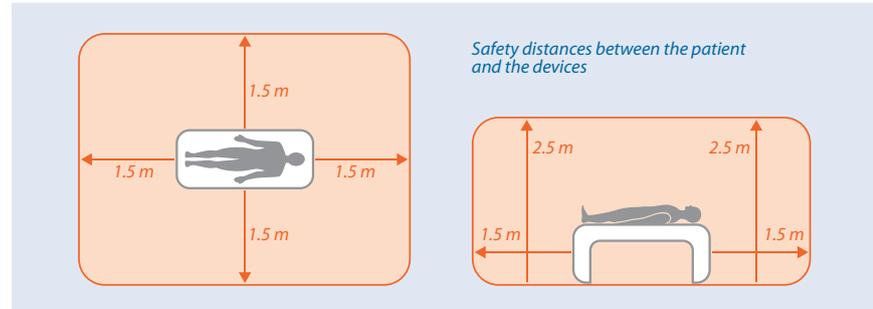
Without medical safety devices, e.g. medical protector, the PC and all non-medical connected instruments (e.g. monitor and printer) of the system must be installed and operated in a distance of at least 1.5 m to the patient seat (see orange area in the illustration) because leakage current might occur.
