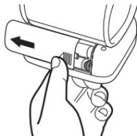
Pressing down on the battery cover, slide the cover off in the direction of the arrow.
