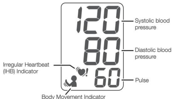
The Body Movement Indicator is displayed on the measurement results display if you move your hand or wrist during measurement, causing a substantial pressure change to be detected.
