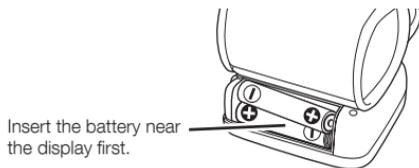
Insert the battery near the display first.
