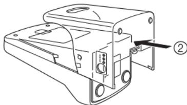
**HOW TO UNLOAD THE BATTERIES****1 Remove the plug, pocket and battery compartment cover.**
