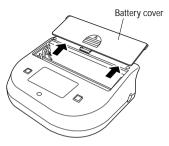
Remove the battery cover at mainframe and replace four type "AA" batteries.
