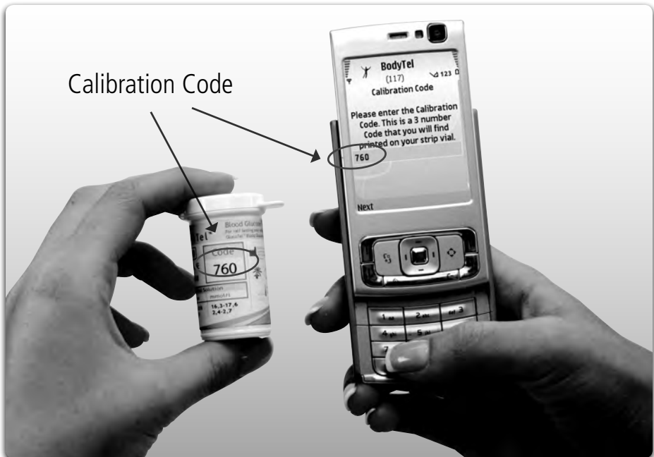
Fig. 3 – Calibrating your GlucoTel Meter. Example shows Calibration Code #760.
