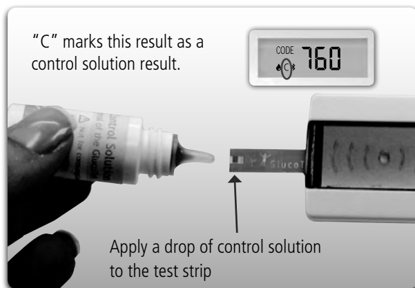
Fig. 4. Applying Control Solution to GlucoTel Test Strip
