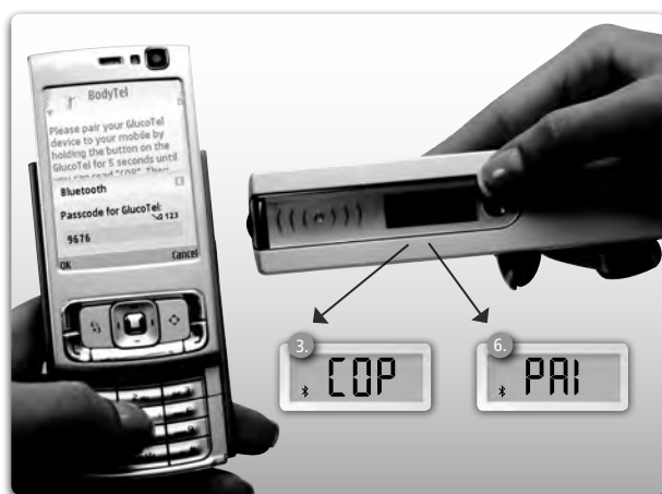
Fig. 2 Pairing the GlucoTel to your Mobile Phone – hold the devices near one another while pairing.
