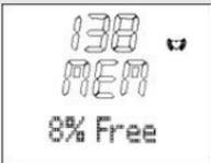
The message shows '138' on the top line, 'MEM' on the second line, and '8% Free' on the third line. A small arrow icon is to the right of the top line. | During training, the HR watch signals every 5 seconds <b>MEM x% Free</b> , if less than 10% of the memory is free.<br>On the display: <b>MEM 8% Free</b> (still 8% free).               |
