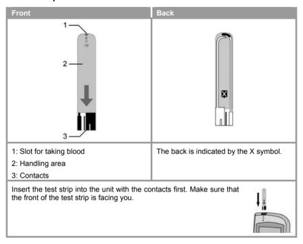
Read carefully the following information on the handling and storage of your test strips. All instructions must be followed to ensure that the test strips will give accurate test results.
