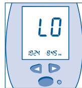
Blood Glucose Test Lower Than 20 mg/dL
