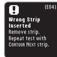
A strip error displays if a used strip is inserted, the strip is inserted upside down, or the wrong strip is inserted.
