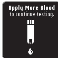
If the first blood drop is not enough, the meter will beep twice and display **“Apply More Blood to continue testing.”** You have about 30 seconds to apply more blood onto the same strip.
