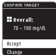
5. A screen then shows the current Target settings. Press the **OK** button to **Accept** these Target ranges. To change the Target range, highlight **Change** and press the **OK** button. **Set Target** will be highlighted. To set targets, see the Target setup section on the following page.
