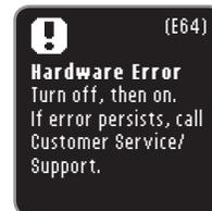
A system error displays when either the meter software or hardware malfunctions.
