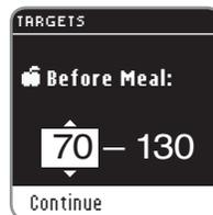
11. Use the ▲ or ▼ button to change the highlighted Before Meal Target value. When you see the Target value you want, press the **OK** button, and you will move to the next Target value.
