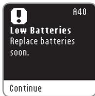
When the batteries are low, the **Low Batteries** screen displays. Press the **OK** button to acknowledge the warning. The system continues to operate normally, but the low batteries icon appears on the Main menu until the batteries are replaced. Change the batteries right away. You may only test about 10 more times over the next three days before the batteries run out.
