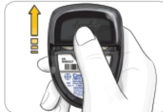
Turn off your meter before changing your batteries. Press firmly on the battery cover and slide in the direction of the arrow.
