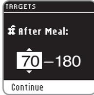
16. Use the ▲ or ▼ button to change the Target value. When you see the Target value you want, press the **OK** button, and you will move to the next Target value. Press the **OK** button when you are finished.
