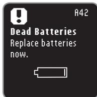
When you are no longer able to perform a test due to low batteries, the **Dead Batteries** screen will show. Change the batteries immediately.
