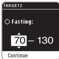
6. Use the ▲ or ▼ button to change the highlighted value. When you see the value you want, press the **OK** button, and you will move to the next Fasting Target value (130 mg/dL).
