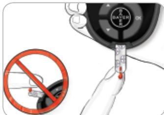
4. Immediately touch the tip of the test strip to the drop of blood. The blood is pulled into the test strip through the tip.
