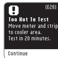
A testing condition error displays when the meter is too cold or too hot to test.
