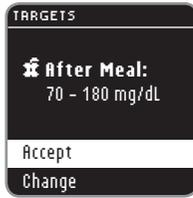
14. The After Meal Target range will appear (70 - 180 mg/dL). You can **Accept** the highlighted Target by pressing the **OK** button.
