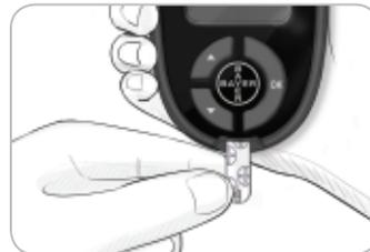
3. Insert the gray square end firmly into the test strip port until the meter beeps.
