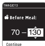
12. To change the Target, use the ▲ or ▼ button and press the **OK** button when you are finished.
