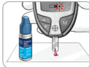
7. Squeeze a small drop of solution onto a clean, nonabsorbent surface.
