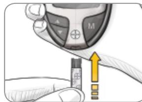
3. Hold the test strip with the gray end facing up.
