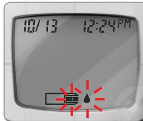
The meter will turn on. An image of a test strip with a flashing blood drop will appear letting you know the meter is ready to test.
