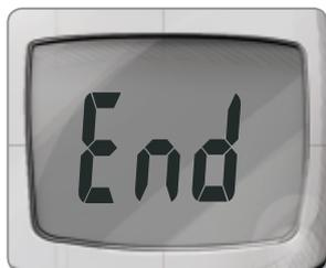
Press ▲ again and you will see **End**. Press **M** to turn the meter off, or it will automatically turn off after 3 minutes.
