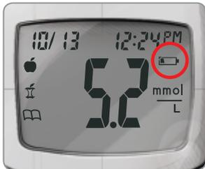
Batteries should be replaced when the meter continually displays
