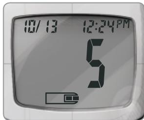
You will see the meter count down 5 seconds until the test is complete and your control test result is displayed.
