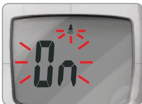
The flashing bell symbol will now appear on the display along with the word **On**.
