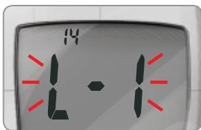
After setting the sound, **L-1** will flash. To keep your meter in Basic Mode, press **M** to set. To change your meter to Advanced Mode, press **▲** or **▼** to change to **L-2**, and press **M** to set.
