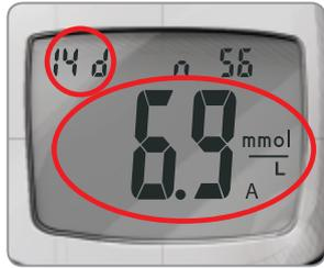
The **14 day average** will appear in the center of the display with the number of results shown at the top of the display. Any control results are not included in this 14 day average.
