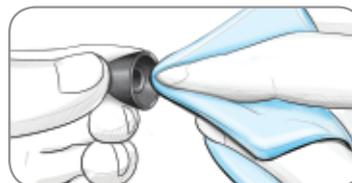
3. Using a new germicidal wipe, carefully wipe all external and internal surfaces of the endcap until wet.
