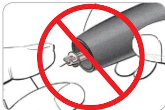
1. Do not use your fingers to remove the lancet from the lancing device. Your Bayer device has an automatic lancet ejection feature.
