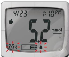
When the reminder sounds, the meter will automatically turn on. The reminder will beep 20 times, and the display will show the pre-meal test result you marked when you set the reminder. Pressing any button will silence the reminder.
