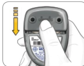
5. Slide the battery cover back into place, lining up with the open slots, and close firmly.
