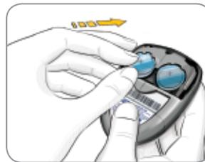
4. Place new batteries under the prongs and into the battery compartment with the “+” side up. [Use two 3-volt (DL2032 or CR2032) lithium batteries.]
