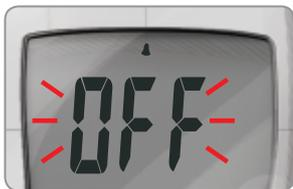
To turn the beep sound off during testing, press **▲** or **▼** to display **OFF**.
