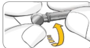
2. Loosen the round protective cap on a lancet by rotating it  $\frac{1}{4}$  turn, but do not remove it.
