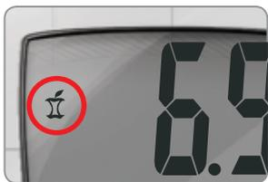
When you have completed this test and the result is shown on the display,  $\bar{I}$  will flash. To mark this test as a post-meal result, press **M**.
