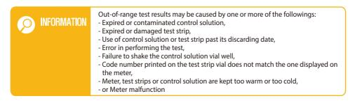
If your control solution test results continue to fall outside the range printed on the test strip vial, the GlucoDr Blood Glucose Monitoring System may not be working properly.
