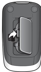
**[2] Remove and Install the Meter Battery:** To remove the used battery, pull the appropriate tab to pop out the battery. Install the new battery with the positive (+) sign facing up towards you.
