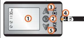
[1] **Display:** Glucose test results, symbols, messages, and graphs appear here. [2] **CENTER Button:** Use the CENTER button to confirm an option or make a selection in a menu. [3] **RIGHT Arrow Button:** Use the RIGHT arrow button to scroll forward through options. [4] **Strip Port:** Insert the WaveSense KeyNote Test Strip, with the contact bars facing up, into the strip port. [5] **LEFT Arrow Button:** Use the LEFT arrow button to scroll backward through options.
