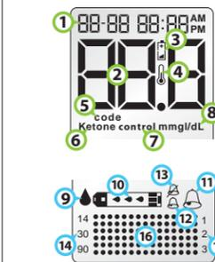
[9] **Apply Sample to Test Strip:** The test strip symbol and flashing droplet symbol will signal you to apply sample to the test strip. [10] **Sample Entering Test Strip:** The three droplet symbols will appear within the test strip symbol when blood or control solution enters the test strip. [11] **High Volume:** large bell indicates
