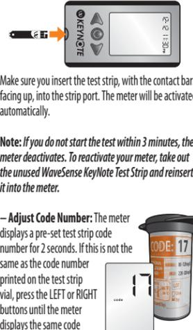
number as printed on the test strip vial. The meter now displays the blood drop and test strip symbols. The WaveSense KeyNote System is now ready for you to apply blood.
